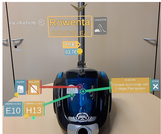
Figure 3: Comparison view of a product within the “filtration” category. Attributes linked to physical parts are attached to them through a line with a circled end.
